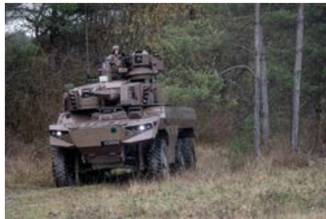
Jaguar: French armoured reconnaissance vehicle. It has a 40 mm gun and carries two anti-tank missiles. © Armée de Terre française
