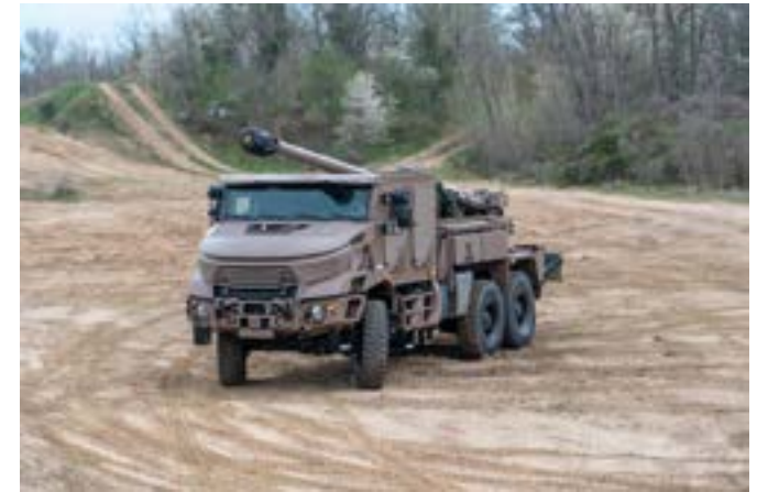
Caesar is a French wheeled, 155 mm 52 calibre self propelled howitzer. It holds 18 rounds and is typically operated by a crew of five, though if necessary can be operated by a crew of three. It can be transported by a C-130 or an A400M aircraft. France has ordered 109 more Caesars having gifted a significant number to Ukraine. Authorised by KNDS
