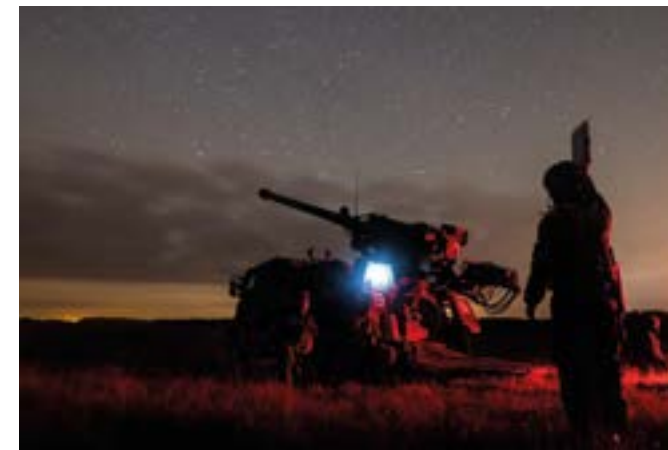
The French Caesar 155mm/52 calibre gun. With an unassisted range of around 40km, the gun delivers both General Support and Close Support tasks and can support the DRF as well as the manoeuvre brigades. The range is as important for depth as it is for enfilade in order to mass trajectories in the close battle. nexter.mourmelon
